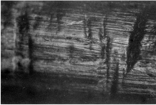
Fig. 2 Wear formed experimentally by punching holes in leather (100X magnification)
